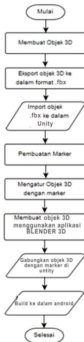
Gambar 3. Diagram alur Augmented Reality
