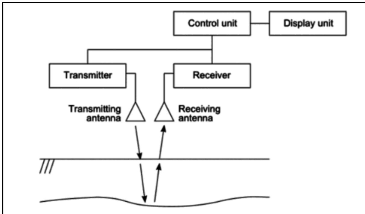
**Figure 2.** Basic Principles of the GPR Method (Takahashi et al, 2013)
