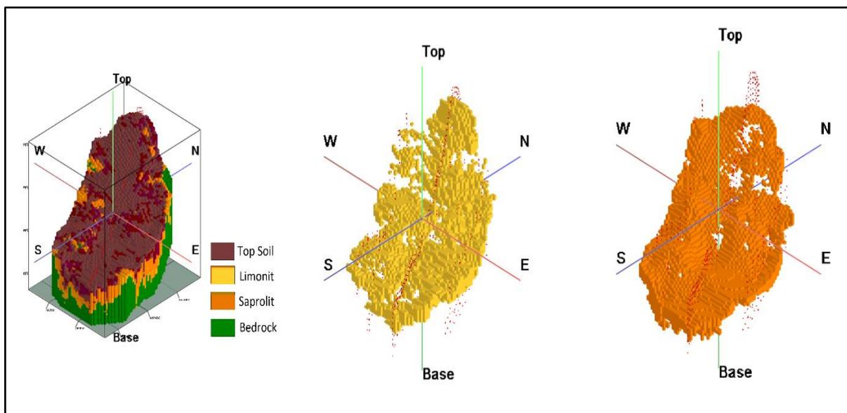
**Figure 7.** 3D Model of (a) Nickel Laterite Deposits (b) Limonite Layers (c) Saprolite Layers
