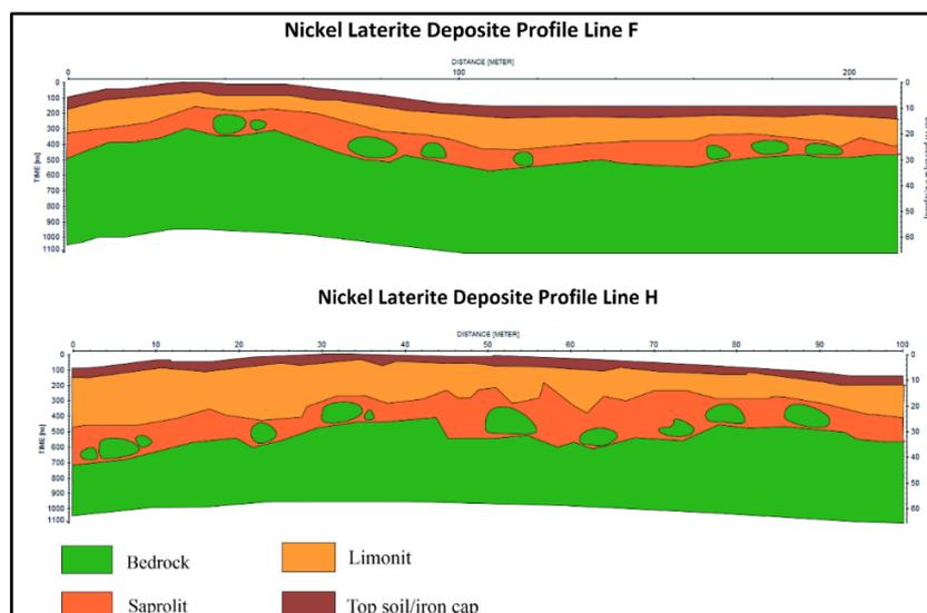
**Figure 5.** Nickel Laterite Profiles of Line F and H
