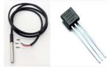
Gambar 4. Sensor Suhu DS18B20
