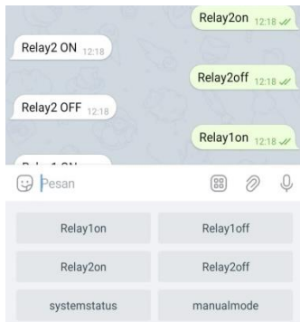
Gambar 16. Perintah Manual Relay 1 Relay 2 ON dan OFF
