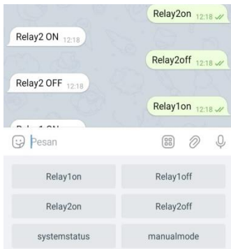
Gambar 16. Perintah Manual Relay 1 Relay 2 ON dan OFF
