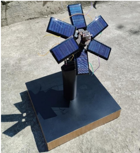
Gambar. 3 Hasil Rancang bangun Sunflower Solar Tracking
