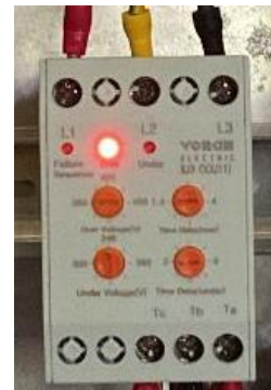
Gambar 10. Pengujian Phase Failure Relay Keadaan Over
