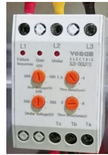
Gambar 9. Pengujian Phase Failure Relay Keadaan Normal
