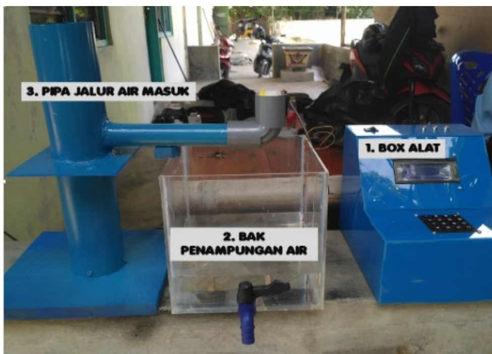
Gambar 9. Purwarupa sistem monitoring kondisi air
