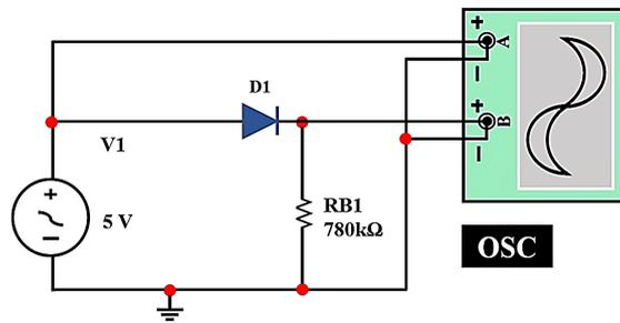
Figure 3. Half-wave rectifier circuit diagram. Source: [13]
