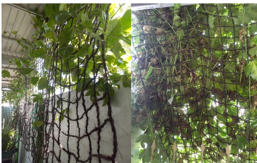
Figure 10. The AP ropes and nets under viners load.
