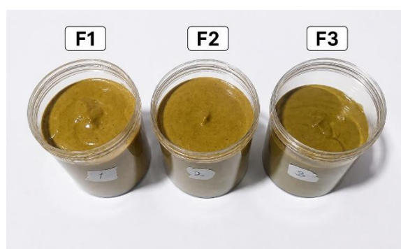
Figure 1. Representative appearance of kepunding leaf ethanol-extract creams (F1-F3) showing homogeneous texture and no visible phase separation during 14-day storage at 25°C
